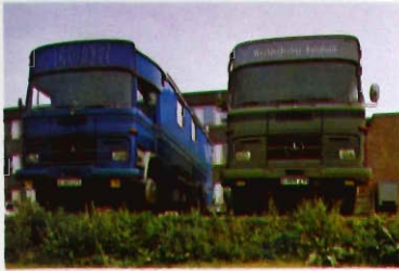
Two WDR Outside Broadcast units. On the left a 3-camera bus, on the right a special, VTR van.
