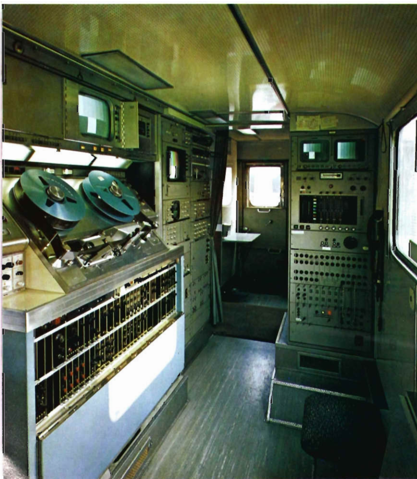
TR-70's take to the road in WDR OB unit to telecast/record a wide range of outdoor and remote events.
